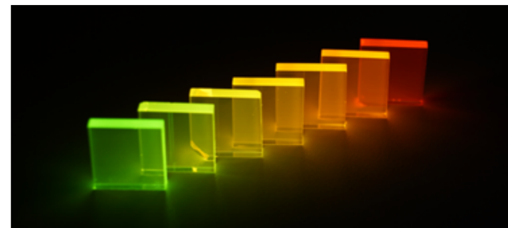
Luminescent glasses enriched with various metal ions under excitation with ultraviolet light.
