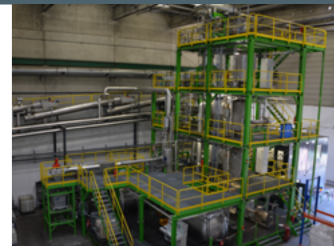
CARBOLIQ pilot system for oiling of alternative fuels gained from domestic and industrial waste in the Ennigerloh disposal center.
